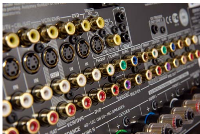
Figure 2: Typical AVR Back Panel
